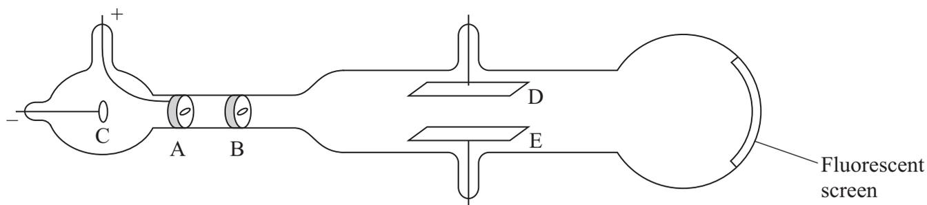
A metal disc at C emits electrons. A positively-charged disc at A accelerates the electrons along the tube. Slits in A and B produce a narrow horizontal beam of electrons. An electric field is produced between plates D and E, which can be used to deflect the beam vertically. The final position of the beam is shown on a fluorescent screen at the end of the tube.
